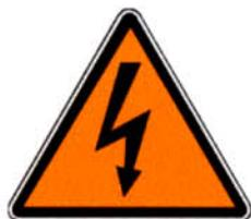
The lightening flash with arrow head symbol within an equilateral triangle is intended to alert the user to the presence of dangerous voltages and energy levels within the product's enclosure that may be of sufficient magnitude to constitute a risk of electric shock or injury.
